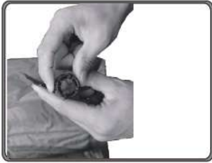
1.Unscrew the gas nozzle counterclockwise.
